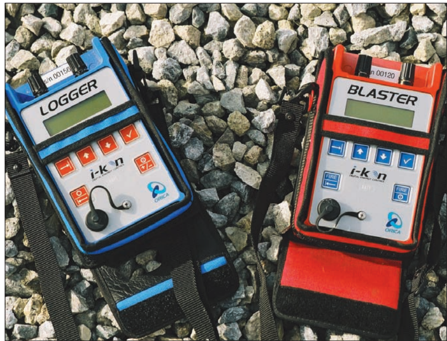
i-kon® electronic technology controls the way a series of explosions interrelate, with precisely timed delays ranging from a few milliseconds to several seconds
