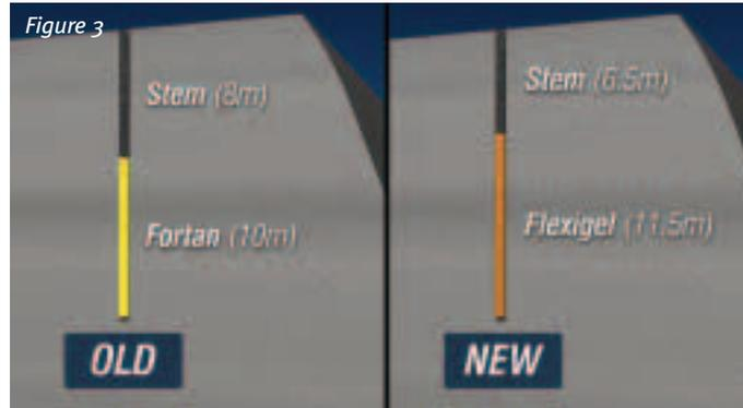
Orica took over management of the drill and blast operations and following a full assessment developed 18 distinct templates. The result was a greater than 30% improvement in production at a lower overall powder factor.
