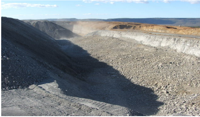
Picture 2: Eastern Creek ABT post blast profile
