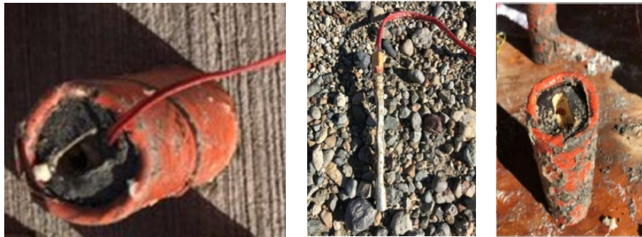
Figure 1: Dynamic pressure misfires can often not be identified until the detonator is removed from the booster
