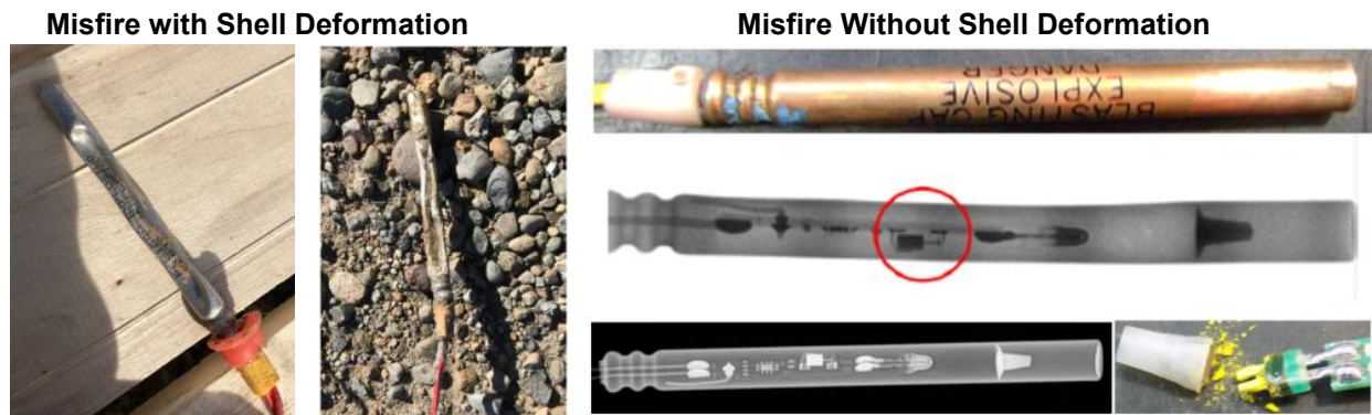
Figure 1: Misfires caused by dynamic pressure, can occur both with and without obvious external shell deformation.
