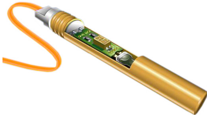
Cut-away view of an i-kon™ Detonator VS
